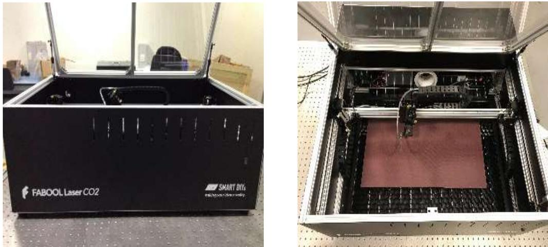
Figure 3.2: CO<sub>2</sub> FABOOL Laser Mini
